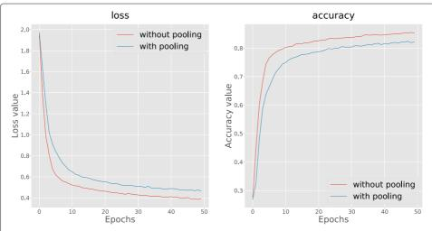
**Fig. 18** The loss and accuracy are from the first 50 epochs between using the max-pooling layer and without using the max-pooling layer
